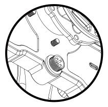
Alternatively, you can use the aviation connector located at the back of the product
