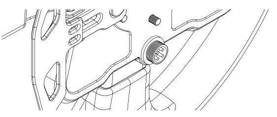
If you are using the aviation connector, please connect the MX1.25 6-pin connector on the aviation connector to the socket on the PCB
