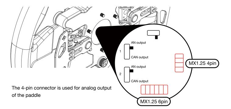
The two switches on the left side represent the output modes for the two paddles
