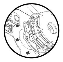
You can use any quick-release wiring connector that allows for cable pass-through (Zestek quick -release)
