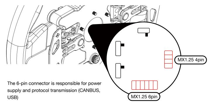
Typically, the connector wiring definitions are printed on the PCB surface
