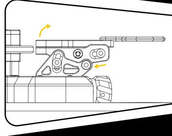
Loosing the screws on the back to adjust the distance between the pedals and the edge of the steering wheel, which allows OEM HUB to support the steering wheels from 310 to 350.
