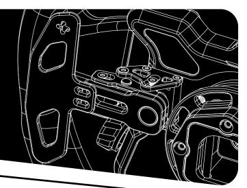
Loosen four screws on the left to adjust the distance between hands and pedals.
